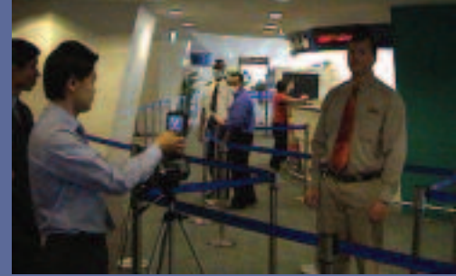
Setting up a ThermaCAM™ P60 with Automatic Temperature Compensator (ATC) at Singapore Cruise Centre.
