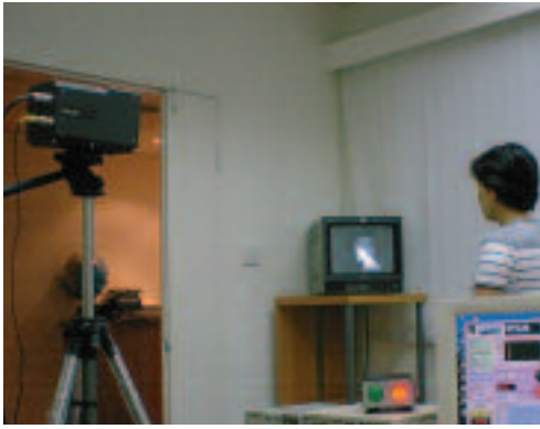
First experimental set-up in the lab. The FLIR Systems IR camera is set to generate both a colour, visible and audible alarm.
